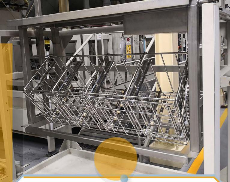
We develop and manufacture customer - specific bogies and rotary trommels with individuell size and request for usage in cleaning or coating systems. Depending on the loading weight, sheet metal and wire combinations form the basis of our developments.
