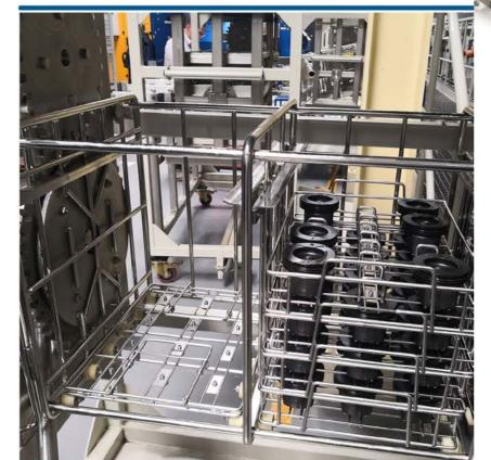
Thanks to the optimized bogie, media and washing mechanics, for example ultrasound or spray jet, reach the items to be cleaned from all sides. This not only contributes to an improved cleaning quality, but also noticeably extends the service
